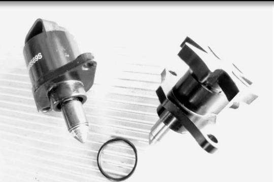
8 / Reinstall the new O-Ring ( it has been coated with silicone grease).
