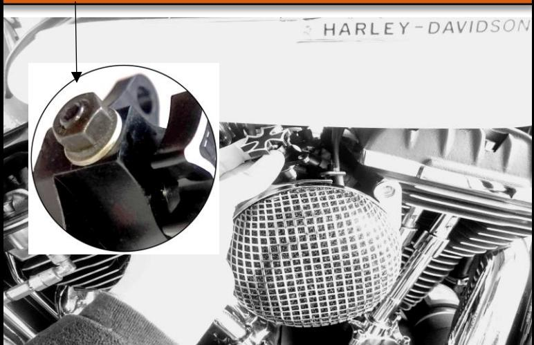
10 / Unscrew the "Wheel knob " upwards BEFORE bolting!
