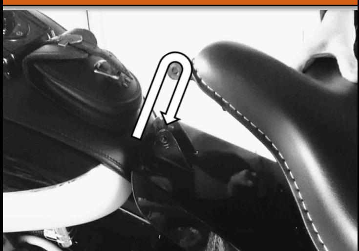
Before starting your VTwin, make sure that the adjustment knob is unscrewed upwards and then back by 2 to 3 X  $\frac{1}{4}$  turn.
