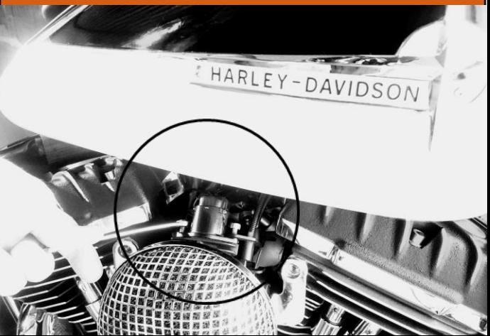
5 / Unplug the plug & remove the servomotor
